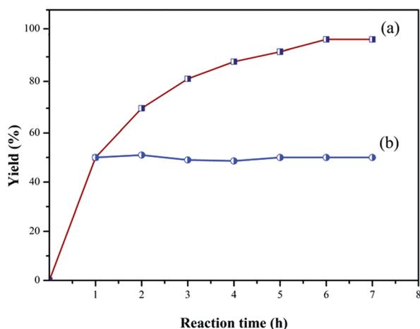
Fig. 4 (a) The kinetic plot of hydrogenation of 4-nitropyridine; and (b) the reaction kinetics when the catalyst NAP-Mg-Pd(0)PS was removed from the reaction mixture after 1 h.
