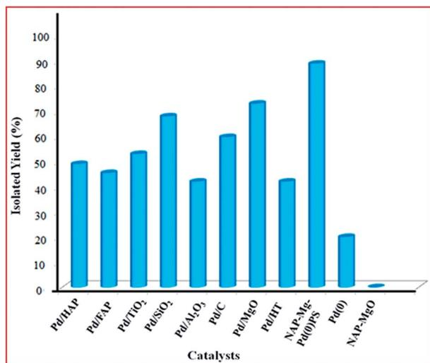
**Fig. 2** Hydrogenation of 4-nitropyridine using various Pd catalysts. <sup>a</sup>Reaction conditions: 4-nitropyridine (1.0 mmol), catalyst (0.020 g, Pd: 1.98 mol%), Et<sub>3</sub>N (0.75 mmol), PMHS (4 mmol), H<sub>2</sub>O (3 mL), 80 °C, 6 h.
