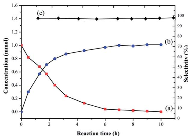
Fig. 3 Hydrogenation of 4-nitropyridine: (a) concentration of 4-nitropyridine; (b) concentration of 4-aminopyridine; (c) selectivity of 4-aminopyridine at different reaction times.
