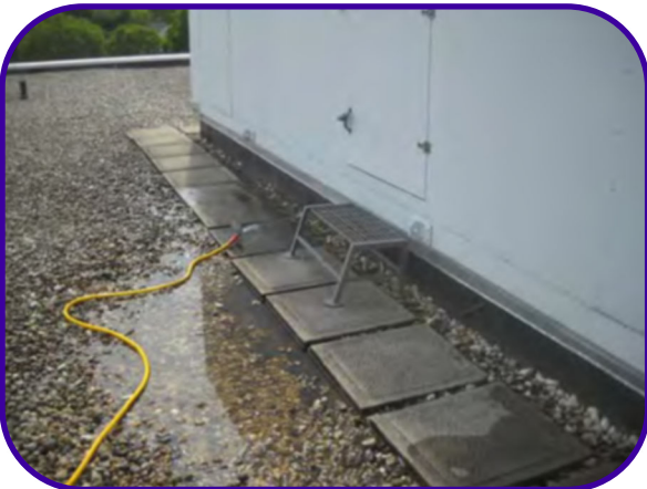
Water Test Area #2 – Location of moisture infiltration is at a pipe penetration located just inside and to the right of the penthouse door
